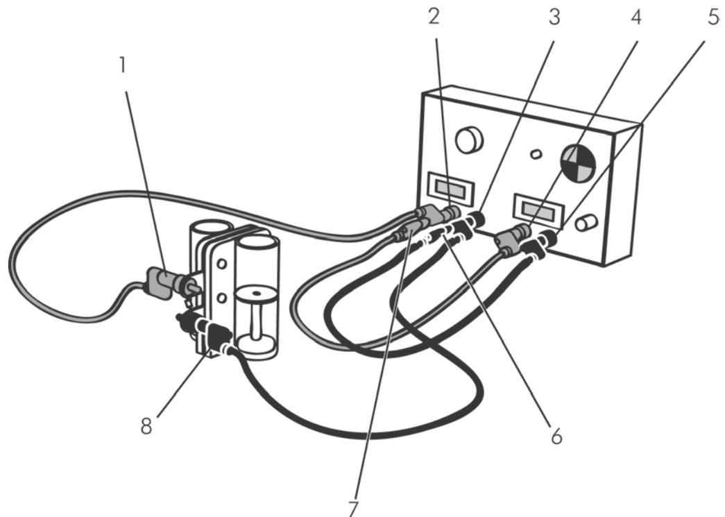
Fig. 4-1 Connecting the reversible fuel cell with the load measurement box
