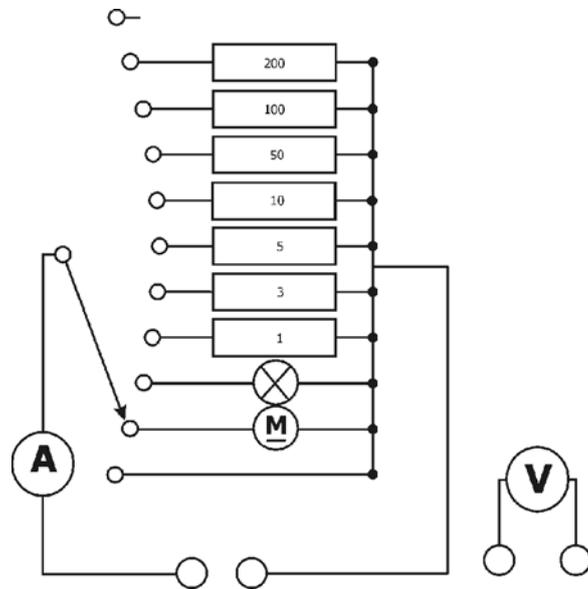
Fig. 6-1 Wiring of the load measurement box
