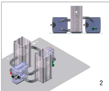
4. Fit caps to the bottom connectors of the fuel cell (Fig. 2).
