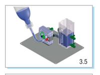
8. Attach the water bottle to the bottom connector on the oxygen side of the RFC with the included tubing (Fig. 3.5).
