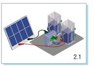
Use the cables to connect the solar module to the appropriate terminals on the RFC. When doing so, make sure that the polarity is correct (red = "+", black = "-"). The cell will begin to produce hydrogen and oxygen in a 2:1 ratio (Fig. 2.1).
